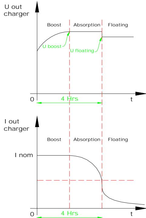
Boost Phase: starts up automatically when the charger is turned on if the battery is flat. The current is then at maximum output.
